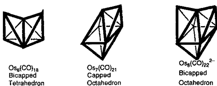
Fig. 4. Examples of chemically significant polyhedra with tetrahedral chambers: all of these polyhedra are found in osmium carbonyl derivatives.
