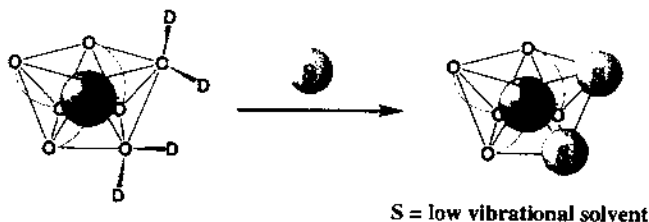
Fig. 8. Suppression of energy transfer quenching via vibrational excitation by replacing coordinated \text{D}_2\text{O} molecules by low vibrational solvent molecules.
