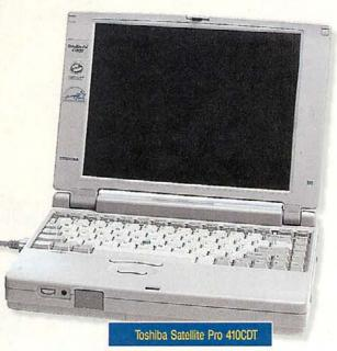
the floppy in place of the CD-ROM drive. (The Toshiba was the only unit that allowed us to swap the CD and floppy without rebooting. Just put the notebook into suspend mode, swap the drives, then turn it back on and pick up where you left off.)
