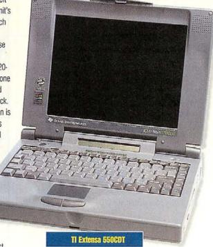
Equipped with a 75-MHz Pentium processor, 256K L2 cache, PCI localbus video, and 16-bit sound, this value-line unit offers snappy, if not blazing, performance.
