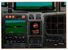
DESIGNATED HITTER The independent thermal viewer enables the commander to designate targets for the gunner. The multifunction display records the relative positions of friendly and enemy units.
