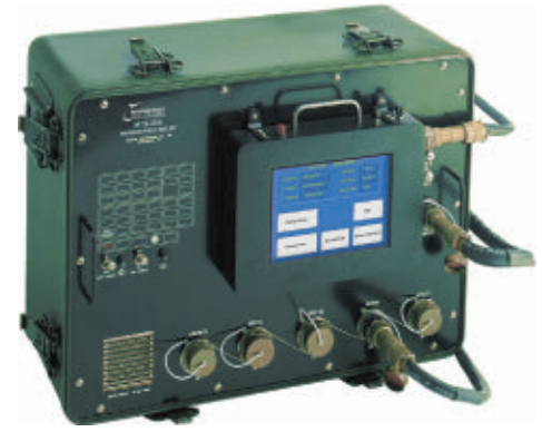
Figure 2. Marvin Test Solutions collaborated with the United States Air Force to create the modern, portable flightline test set for the A-10/C Thunderbolt II.
