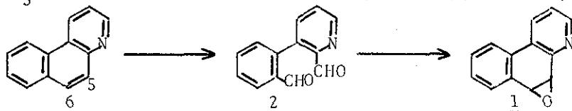
As reactions of the epoxide(1), an acid catalyzed isomerization to phenol, nucleophilic additions of hydroxide and methoxide, and a photochemical reaction were examined.
