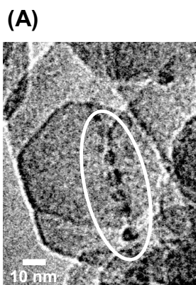
Figure 2. (A) TEM image of CuHT(c); (B) Size distribution diagram for the Cu nanoparticles of Cu/HT(c)
