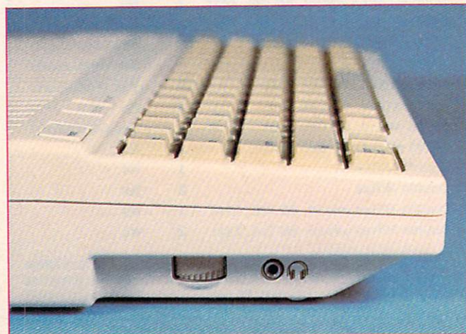
The left front side of the IIc showing the volume control and earphone jack. When earphones are plugged in, the internal speaker is disabled.
