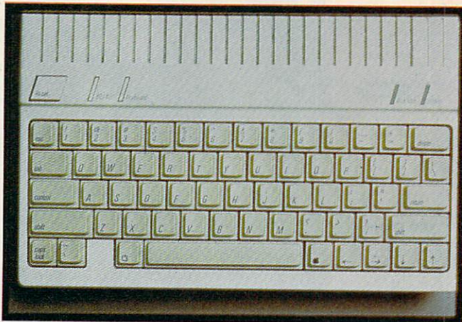
The top of the IIC . Note the reset, 40/80 (column), and keyboard switches on the top left, and the disk use and power indicators on the top right. When the keyboard switch is activated, the Dvorak layout (shown below) is selected.
