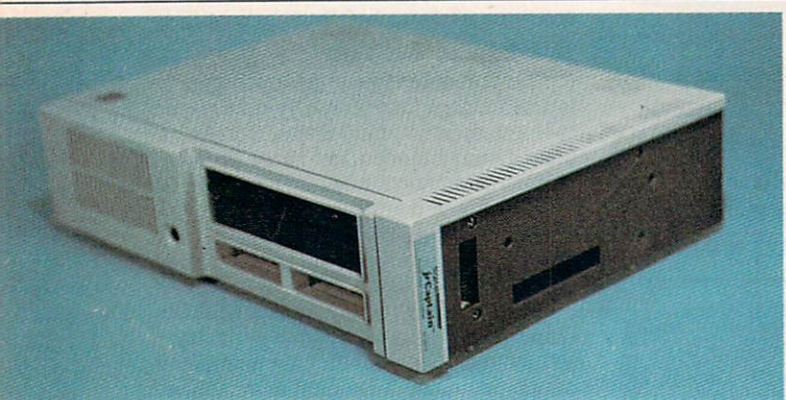
Photo 2: The jrCaptain mounts neatly to the side of the PCjr, just like the the IBM parallel printer port. In fact, it can perform the same functions.
