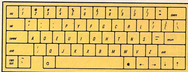
The top of the IIC . Note the reset, 40/80 (column), and keyboard switches on the top left, and the disk use and power indicators on the top right. When the keyboard switch is activated, the Dvorak layout (shown below) is selected.
