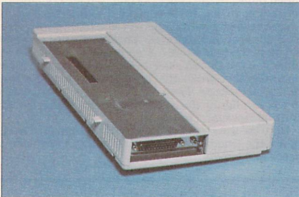
The Side Assembly module has a switch to change from PC mode to PCjr mode. The benefits provided by this switch are uncertain. The connector for the parallel printer port is visible here. This port may be treated the same as the IBM parallel port LPT1.
