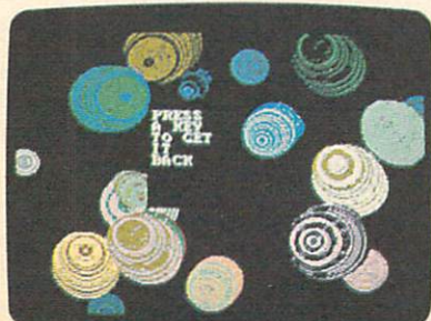
Photo 2. The graphics displaced by the window have been saved in an integer array. When the window is removed, the graphics can be restored to their original condition.
