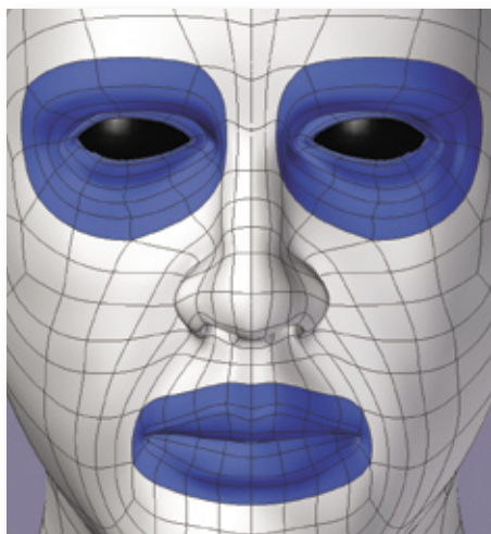
Figure 4—The blue areas on this face represent two common sets of edge loops on a face. The edge loops will help give a natural look to the eyes and mouth when deforming.
