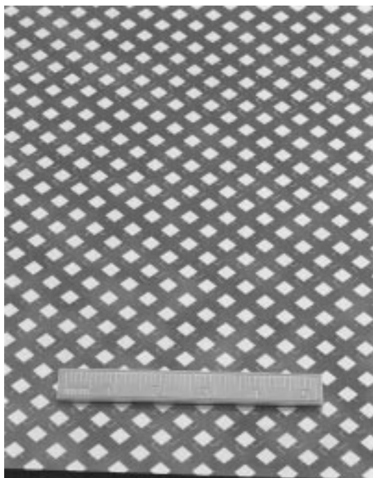
Fig. 8. Close-up view of unit 1 reflectarray showing some elements with phase-delay lines having similar linear dimensions as the patch.
