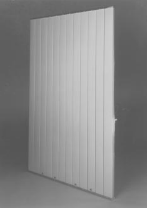
Fig. 1. The 12 × 12 dual-polarized array.
