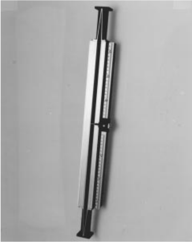
Fig. 3. Photograph of the antenna that was measured in the X -band frequency range. Note the sliding probe and the tapers at each end.
