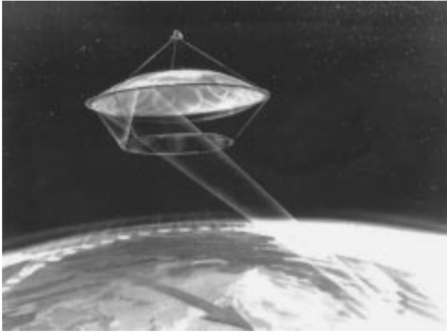
Fig. 2. An artist's rendition of IRIS in orbit around earth. The reflector is an inflatable parabolic torus with a tilt angle of 35^\circ .
