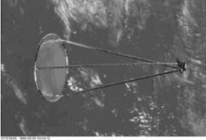
Fig. 10. An inflatable antenna in space (source: NASA Shuttle Web: Electronics still camera photos at website address http://shuttle.nasa.gov/sts-77/images/esc/day2.html ).
