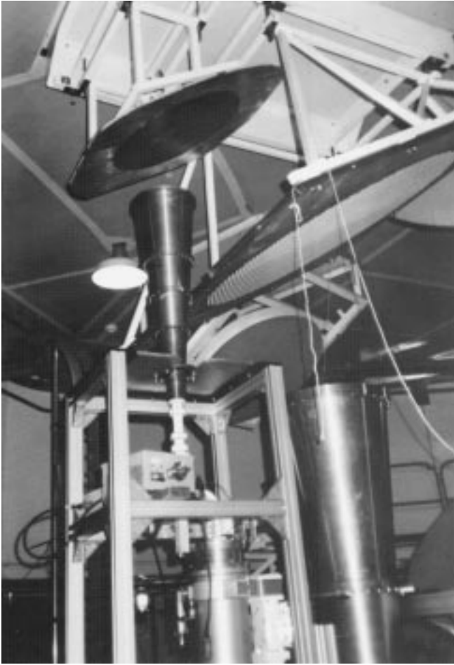
Fig. 12. Feed system installed in BWG antenna.
