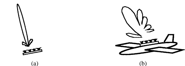
Fig. 1. The radiation pattern of a stand-alone (a) antenna can be dramatically altered by the platform that supports the (b) antenna structure.
