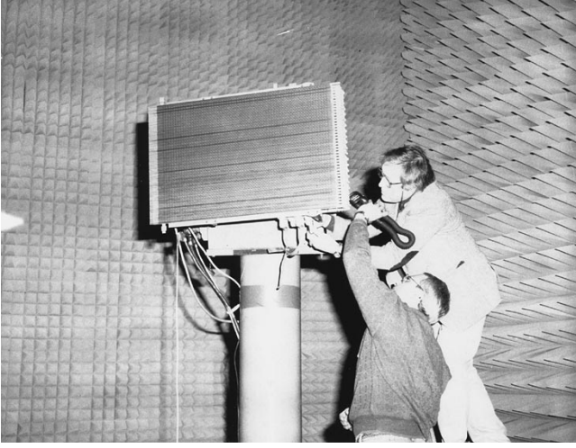
Fig. 6. MSPA antenna aligned for an E -plane pattern in the azimuth plane.
