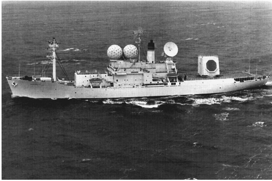
Fig. 4. The COBRA JUDY ship with a clear view of the S -band phased-array and X -band dish-antenna radars.
