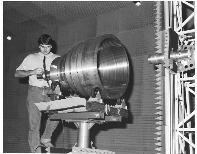
Fig. 5. Photo of the bowl-shaped multihybrid-mode corrugated horn with its linear-polarization input section in the planar near-field anechoic chamber.
