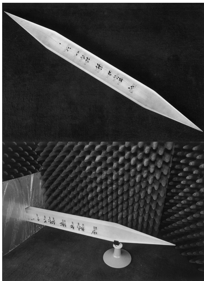
Fig. 2. Photographs of the leaky wave antenna. The dielectric waveguide cross section is 2.75 \times 1.25 inches. The antenna is 36 inches long.
