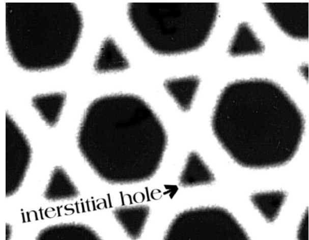
Fig. 6. Magnified view of the cladding region for the HF from Fig. 4.
