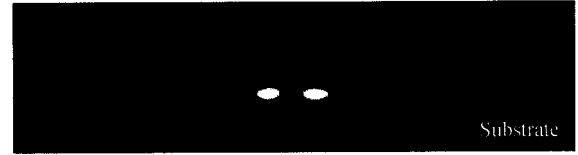
Fig. 7. Near optical field image coming out from the Y-branch waveguide for 1.55 \mu\text{m} light.
