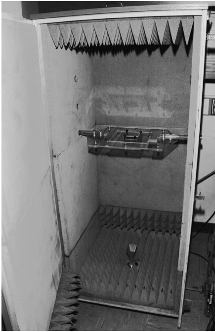
Fig. 7. View of the measurement chamber showing the rectenna panel holder above the transmit horn.
