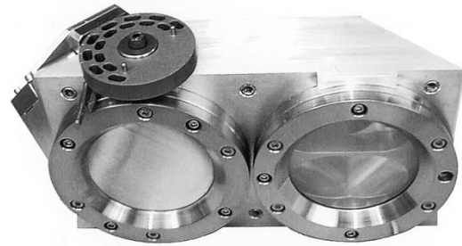
Fig. 4. Polarizing grids mounted on half of the 2.5-THz diplexer. The adjustable path length mechanism is visible in the upper left-hand side. The wheel presses against an invar spacer.
