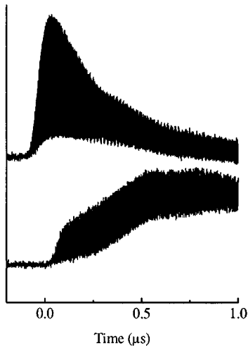
Fig. 11. Optical output of the active-mode-locked laser for B = 0.9 T at \lambda = 97 \mu\text{m} (upper trace) and \lambda = 108 \mu\text{m} (lower trace).
