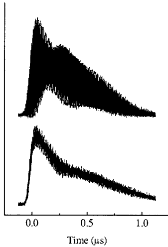
Fig. 10. Optical output of mode locked laser for B = 0.5 T. Upper trace: active mode locking, lower trace: self-mode locking.
