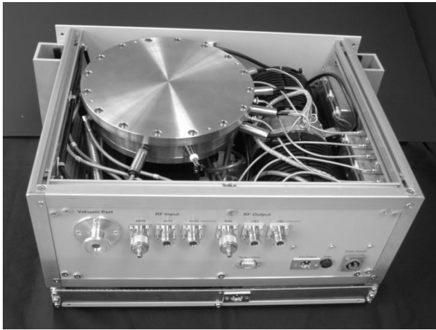
Fig. 13. Demonstrator for a cryogenic BTS receiver front end.
