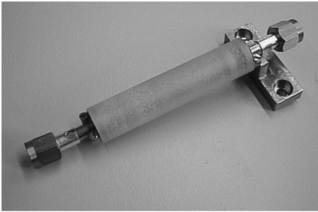
Fig. 9. Cryocoupler for a cryogenic OMUX. The device has an insertion loss of less than 0.03 dB, a thermal resistivity of more than 1000 K/W, and has been tested for power levels up to 200 W.
