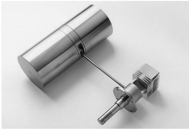
Fig. 19. AIM SL200 cooler, a split Stirling cooler with linear drive compressor. Cooling power 3.5 W@77 K.
