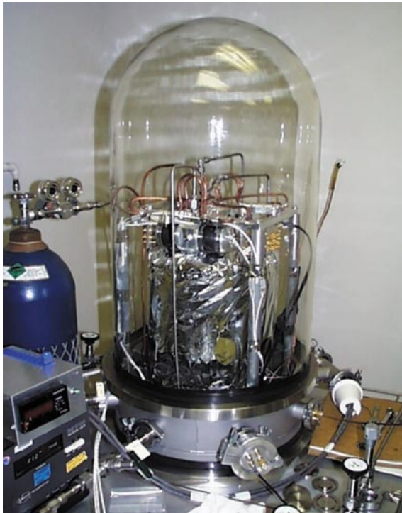
Fig. 9. Sixty-channel HTS input multiplexer and integrated pulse-tube cryocooler inside the vacuum bell jar for testing.
