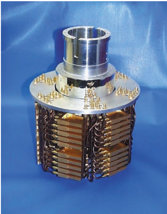
Fig. 6. Sixty filters mounted to the aluminum support structure. Also shown is the fiberglass support tube in place and the cold coax connectors.
