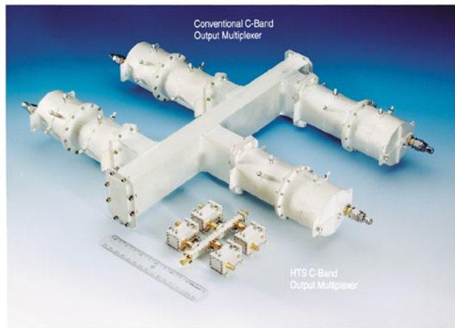
Fig. 2. Comparison between a four-channel superconductive manifold-coupled multiplexer and four-channel C -band output multiplexer built using conventional waveguide technology.
