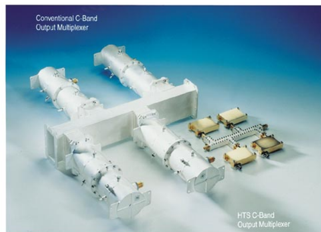
Fig. 10. Layout of a four-channel HTS output multiplexer employing planar HTS filters in comparison of a four-channel waveguide output multiplexer.
