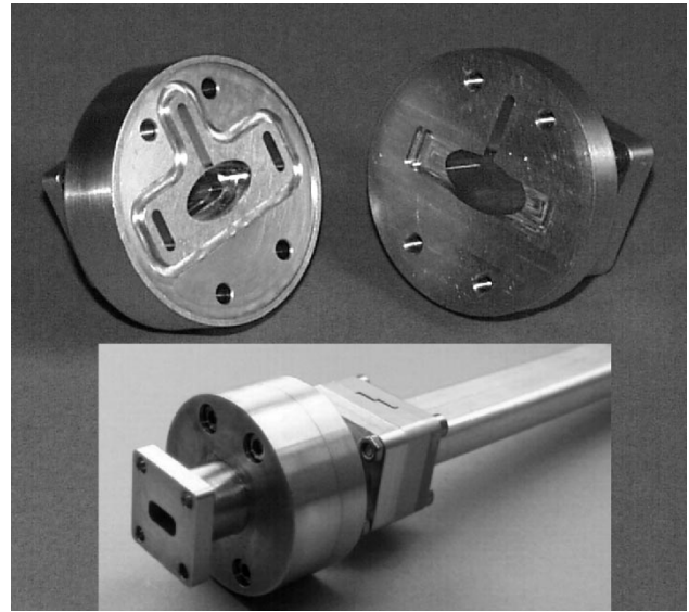
Fig. 5. Two parts of the transition and the transition mounted to the overmoded A185 waveguide.
