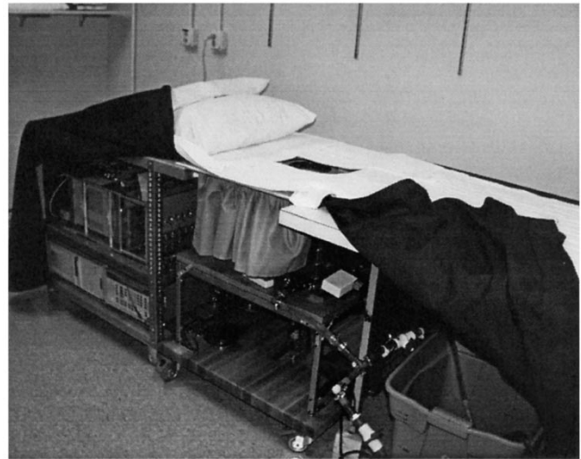
Fig. 3. Fully assembled clinical microwave imaging system with the sheets raised to show microwave electronics and tank overflow reservoir located below the table.
