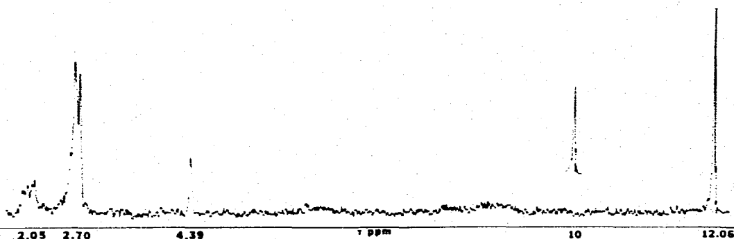
Fig. 1. The proton NMR spectrum of (C_{13}H_9)_2Zr(CH_3)_2 (II) in CCl_4 solution.
