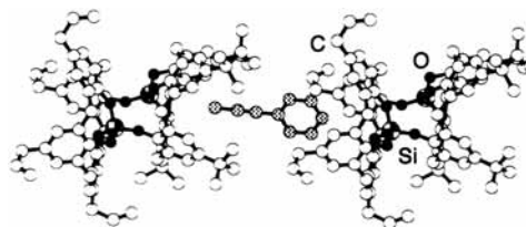
Fig. 8 A portion of the X-ray structure of the inclusion network formed between koiland 5 and phenylpropyne showing the assembling core composed of two consecutive koilands 5 encapsulating a phenylpropyne molecule which acts as the connector. H atoms are omitted for clarity.
