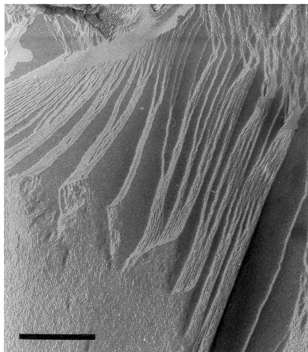
Fig. 3: Typical structure of the lamellar mesophase with 2% (m/m) PHCl observed by transmission electron microscopy (bar = 238 nm).
