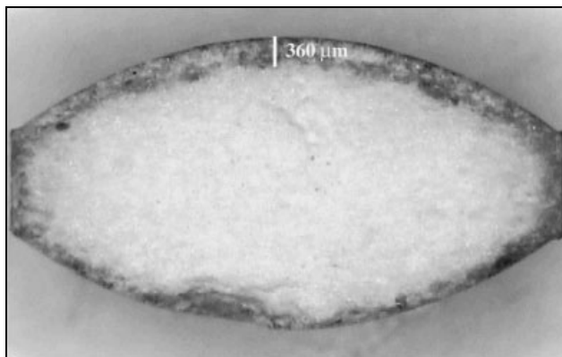
Fig. 8: Cross-section of an irradiated nifedipine 20 mg tablet (Suntest CPS+, 12 h, 720 W/m 2 , UV filter)
