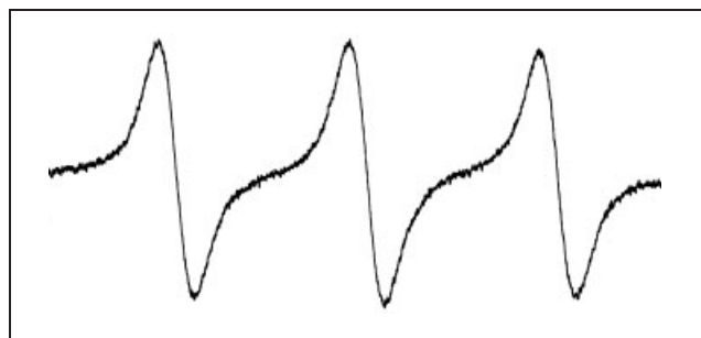
Fig. 1: ESR-spectrum of 1 in methanol at 80 K, mod. 2.5 G, t.c. 100 \mu s, sc.t. 200 s
