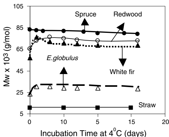
Fig. 4. Effects of incubation at 4 °C on the apparent weight-average molecular weight ( M_w ) of lignins isolated from spruce (black-filled circles), redwood (open circles), white fir (black-filled triangles), E. globulus (open triangles) and straw (black-filled squares). All the lignins were previously completely acetobrominated.
