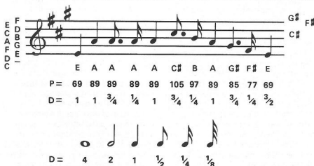
Fig. 5. The first few notes of Hearts of Oak and their digital values for the SOUND command.
