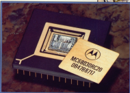
■ Motorola's 68020 microprocessor: the mean, mean number of the 68K family. 'On the fly' it often described as a mainframe on a chip, the processor boasts a clock rate of 25Mhz, instruction and data caches, powerful processing facilities. Barely 160 (in method of speeding up information transmission from main unit) and 68K series compatibility. 4,800 if you want one!
