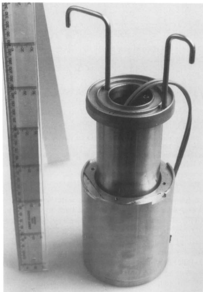
Fig. 2. Photograph of the stainless steel measuring vessel of capacity 1 liter and about 15 cm high. On top of this vessel is the large stainless steel lid (14 cm high) of smaller diameter containing a concentric large surface heat exchanger between incoming and outflowing water. The double flex is connected to the built-in resistor for calibration. The large divisions of the ruler standing to the left measure 5 cm each.
