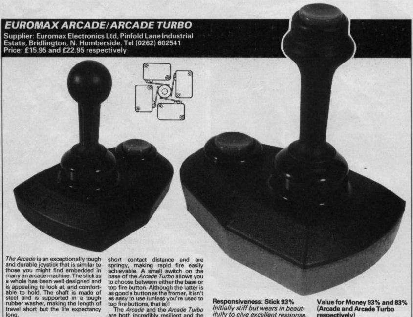
a whole has been well designed and is appealing to look at, and comfortable to hold. The shaft is made of steel and is supported in a tough rubber washer, making the length of travel short but the life expectancy
