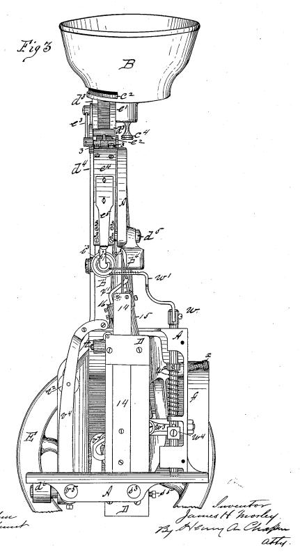
MACHINE FOR SEWING BUTTONS TO FABRICS.
