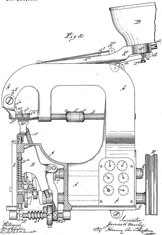
MACHINE FOR SEWING BUTTONS TO FABRICS.
