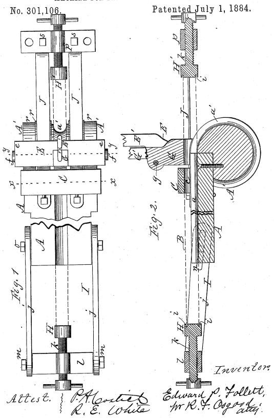
MACHINE FOR BENDING TUBES AND PIPES.
