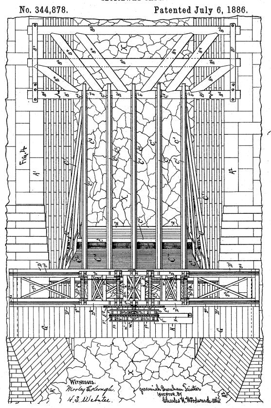
J. B. TAINTER. SLUICEWAY GATE.
