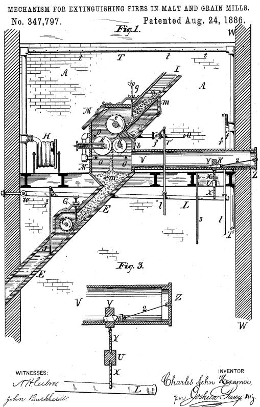
MECHANISM FOR EXTINGUISHING FIRES IN MALT AND GRAIN MILLS.
