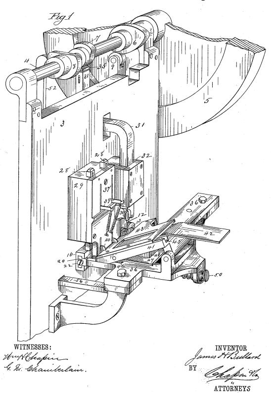
MACHINE FOR BENDING THE ENDS OF KNITTING MACHINE NEEDLES.
