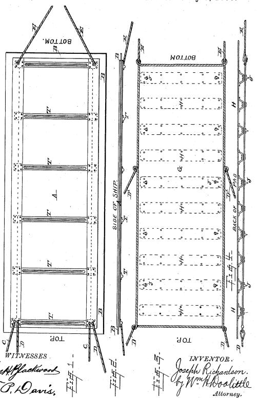
J. RICHARDSON. LEAK STOPPER FOR SHIPS, &c.
