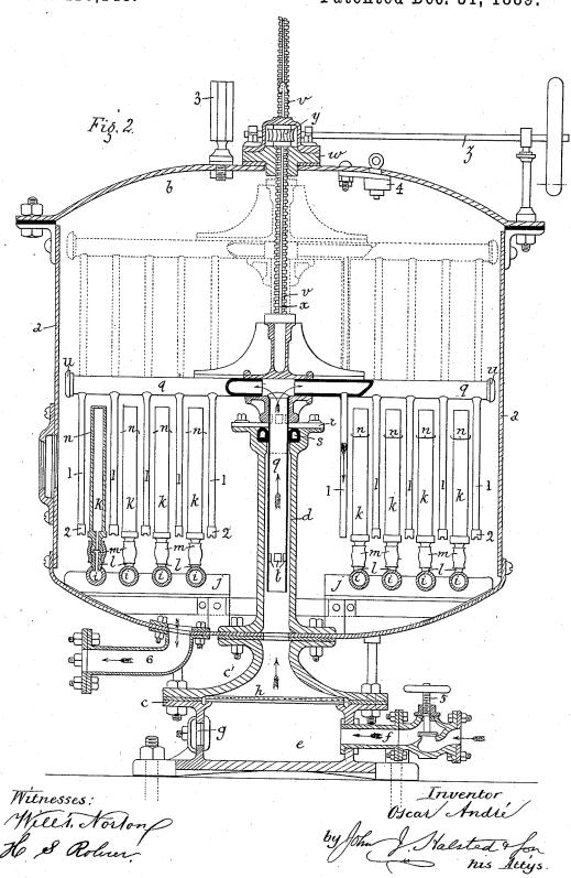
APPARATUS FOR CLEANSING THE BODIES OF FILTERS.
