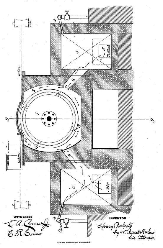
APPARATUS FOR HEATING CONTINUOUS LENGTHS OF RODS, WIRE, WIRE RODS, &c.
