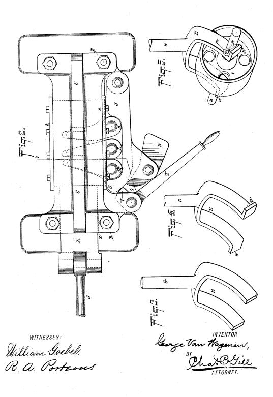
MACHINE FOR THE MANUFACTURE OF WROUGHT METAL SWIVELS. No. 453,751. Patented June 9, 1891.
